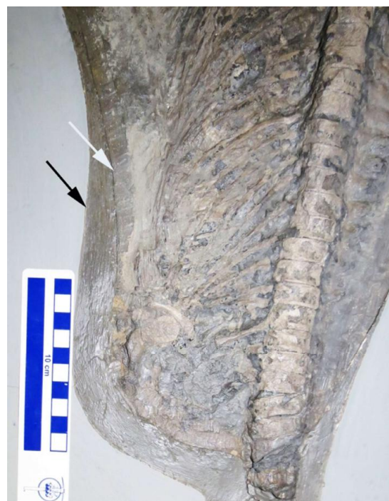
FIGURE 29B: UON VR 159 (TC3199). Closer view of the matrix. White arrow points to outline of genuine matrix and black arrow points to painted 'matrix'. Scale = 10 cm.
